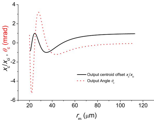
Figure 1: Laser beam parameters at the output of a plasma channel of length 15 mm as a function of matched spot size. Normalized laser centroid offset  $x_c/x_{ci}$  (solid line) and angle (dotted line) are shown for an input centroid offset of  $x_{ci} = 10 \mu\text{m}$ , input injection angle  $\theta_i = 0$ , and  $r_i = 80 \mu\text{m}$ .
