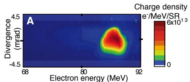
**FIGURE 2.** Electron bunch. The electron energy spectrum of the channeled accelerator shows the appearance of monoenergetic features, here with  $2 \times 10^9$  electrons in a bunch with energy spread of 4% FWHM at 86 MeV. Divergence was near 3 mrad FWHM.
