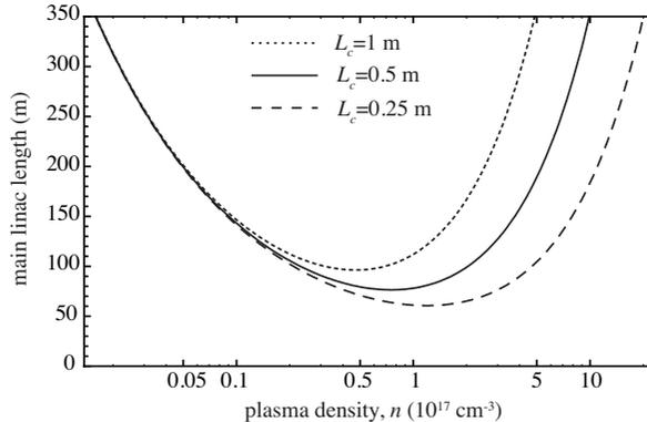
**FIGURE 1.** Main single-linac length versus plasma density  $n_0$  for several laser in-coupling distances  $L_c$ , for  $E_b = 0.5 \text{ TeV}$  and  $a_0 = 1.5$ .
