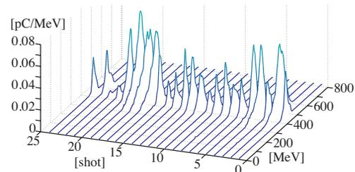
Figure 3: Single shot spectra of 24 consecutive shots for the 33 mm long, 300  $\mu\text{m}$  diameter capillary. (The plasma density was  $\sim 3.4 \times 10^{18} \text{ cm}^{-3}$ , the laser was 1.5 J–46 fs, the applied voltage was 25 kV, and the discharge delay was  $\sim 680$  ns.)
