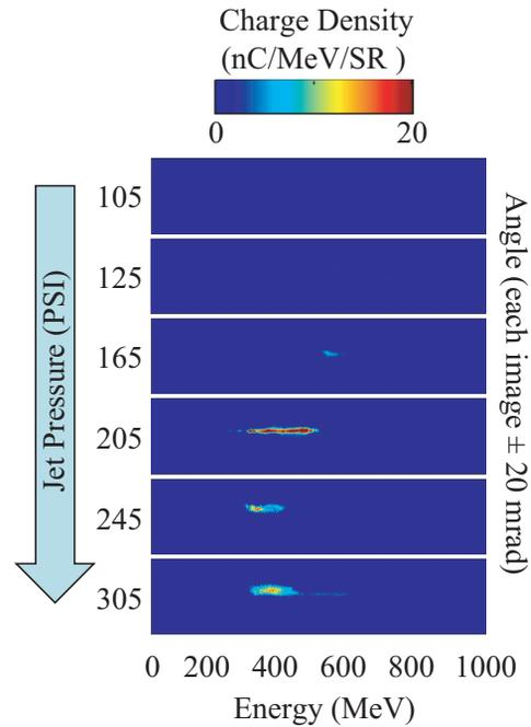
Figure 2: Electron beam spectra as a function of increasing jet pressure for experiments with the smaller jet. The vertical axis is divergence, with extent of each image corresponding to 40 mrad.
