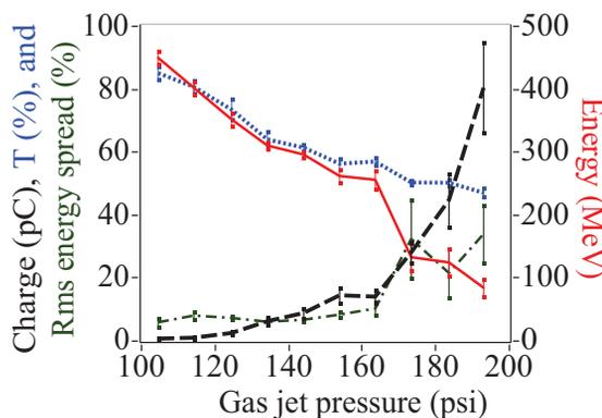
Figure 4: Beam energy (red line, right axis), laser transmission  $T$  (blue dotted line, left axis), integrated energy spread (green dash-dot line, left axis) and charge (black dashed line, left axis) as a function of jet pressure for the larger jet.
