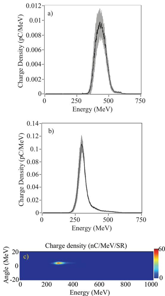
Figure 3: Electron beam spectra for jet pressures of a) 105 psi and b) 145 psi. The black line is the averaged spectrum and the grey shaded area shows the rms shot to shot error for 37 consecutive shots in a) and 26 in b). In c) is shown a sample spectrum for a jet pressure of 145 psi.
