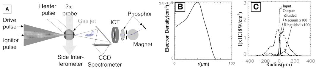
**FIGURE 1.** (a) Experimental setup showing the gas jet with laser beams and diagnostics. (b) The density profile of the channel obtained by Abel inversion of the side interferogram. (c) Mode of the beam at 4TW, showing enhanced transmission with the guide on (unguided modes multiplied by 100 to appear on the same scale). The guided and input modes are similar.
