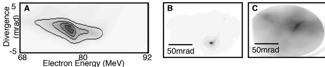
**FIGURE 3.** Electron bunches. The electron energy spectrum of the channeled accelerator (a) shows the appearance of monoenergetic features, here with  $3\text{E}9$  electrons in a bunch with energy spread of 4% FWHM at  $78\text{MeV}$ . Divergence was near 3 mrad FWHM for this bunch (a), and 6 mrad for the whole beam (b). The unguided accelerator in the same gas jet by contrast shows a nearly smooth exponential spectrum with a few MeV temperature (not shown), and much wider divergence (c).
